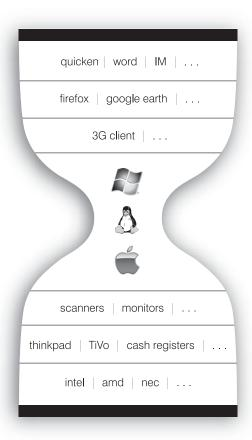
Figure 4.2 Hourglass architecture of the PC
